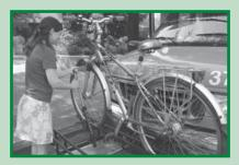
Pull the support arm out and up over the front tire to secure the bike. Use your bike lock to secure the bike to the rack.
