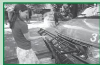
Grab the bar on the front of the bike rack and pull down to unfold.
