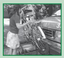
Lift the bike onto the rack, fitting the tires where indicated with marks for front wheels. Use the inside slot (closest to the bus) first.
